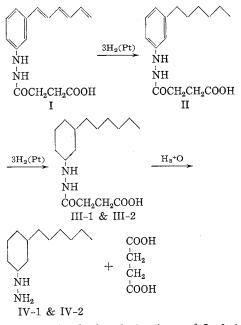
Two dodecahydro-derivatives of I, being detected by thin layer chromatography, are isolated by silica gel chromatography using chloroform-ethyl acetate (1:1) as a developing solvent. A component III-1 is crystallized from chloroform and *n*-hexane. It melts at 97°C. Another component III-2
